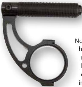
The secondary handle is an easy to fit and versatile accessory which offers additional support and ease of handling when applying torque with Norbar's powered tools. The secondary handle is designed to fit directly to all new powered tools which have a handle location groove in the annulus which is covered by a red rubber band (see inset image to the right).
